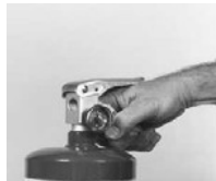
17. Rotate the valve in a clockwise direction until a "click" is heard. This engages threads and minimizes stripping. Hand tighten valve with clockwise rotation.
