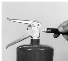
1. Remove the hose assembly or nozzle.
