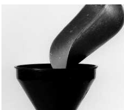
15. Fill the unit with the correct amount and type of dry chemical as stated on the fire extinguisher nameplate. Clean the cylinder threads thoroughly.
