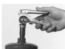
16. Return cleaned valve and syphon tube to the correct cylinder. NOTE: After filling cylinder, replace valve and syphon tube immediately while powder is still in an aerated state.
