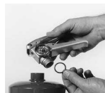
6. Remove body o-ring.
