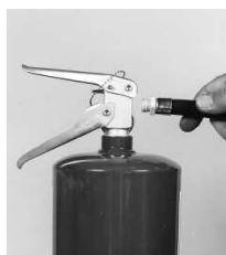
22. Check nozzle and/or hose for blockage and retron to unit.
