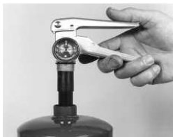
3. Remove the valve and syphon tube from the cylinder by rotating counter clockwise. Mark valve and cylinder if servicing more than one unit. Remove the chemical residue by inverting the cylinder. Failure to do so could result in the packing of powder.
