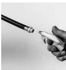
22. Check nozzle and/or hose for blockage and retron to unit.
