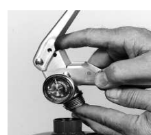
5. Using your finger or a suitable tool, press down on the valve stem located under the discharge handle.
