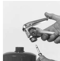
13. Re-insert valve stem assembly into the valve body. Push into place with your finger.
