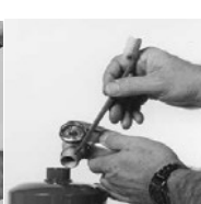
7. With a small brush, thoroughly clean the interior and exterior of the valve body threads, paying particular attention to the seat area. Pay particular attention to the pressure relief groove cut into the threads of the valve body.
