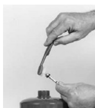
11. Clean the valve seat itself containing the sealing rubber. Strike First recommends replacing the valve stem assembly at every major service interval.
