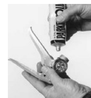
9. Lubricate o-ring circumference. Strike First recommends "Parker O-Lube".
