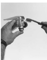
10. Clean outlet orifice with a small brush.
