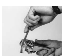
7. With a small brush, thoroughly clean the interior and exterior of the valve body threads, paying particular attention to the seat area. Pay particular attention to the pressure relief groove cut into the threads of the valve body.
