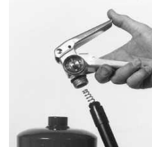
14. Return spring to syphon tube, turn syphon tube clockwise into valve body.
