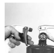
20. Thoroughly chech all areas on the unit that may leak pressure. a) welds b) gauge face & threads c) valve body o-ring d) valve stem seat
