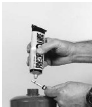
12. Place a small amount of lubricant along the circumference of the small o-ring only.
