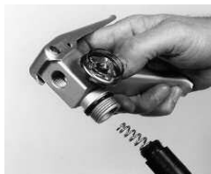
4. Detach syphon tube from valve with counterclockwise rotation. Remove spring.
