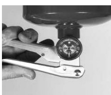
2. Invert extinguisher and discharge all remaining expellent gas.
