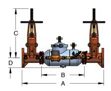
**TYPE 1 BYPASS** 4" DCDALF4A W/ OS&Y GATES SHOWN
